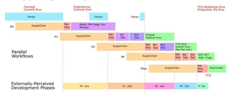
The visible summarized Phases described in the earlier figure are shown at the bottom of the figure just above, to show how detail of the tasks maps to visibility. Here, each Phase is seen to start when its fab steps begin, and continues into key testing defining the purpose of the Phase. Completion of gating tasks enables start of the next Phase, while key testing continues to completion in the current Phase.
