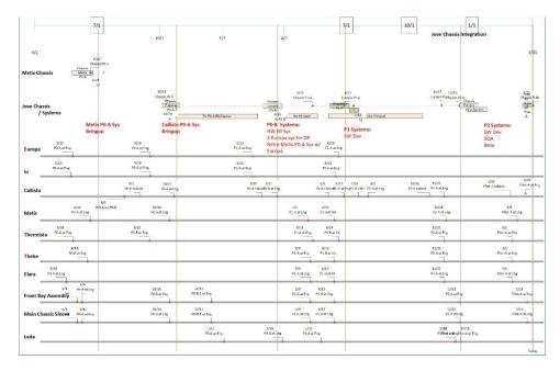
Finally, the full system effort can be shown in perspective and to scale in the following figure. The board-level sub-assemblies at top followed below by system sub-assembly and then by system mechanical structure development.
